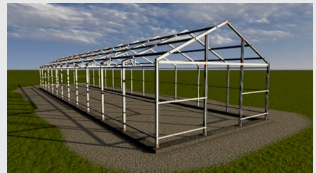
Picture 9: Greenhouse Frame with Steel as the Construction
